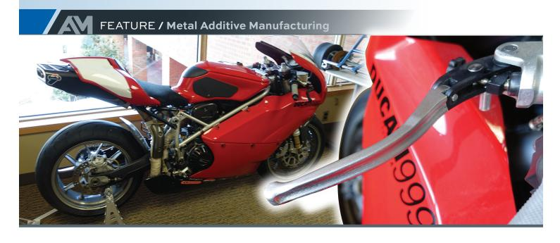
To demonstrate the viability of 3D printing for functional parts, company staff members are replacing one component after another on this Ducati motorcycle with additive parts. Brake and clutch levers have been replaced by one carbon-fiber-reinforced lever made on the composite printer and one stainless lever made on the Metal X.
